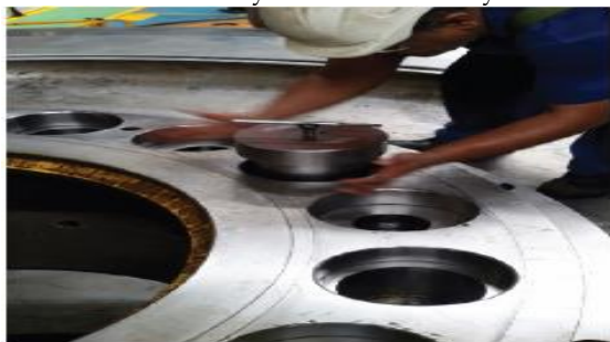
Fig-15 Measurement of coupling flange with template
